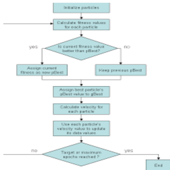
Fig1. Particle Swarm Algorithm Steps
