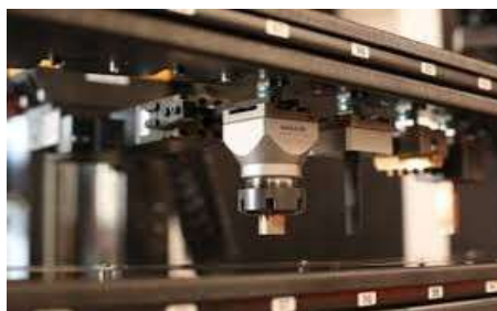
Figure 2. The Electrode setup fixed on the EDM machine
