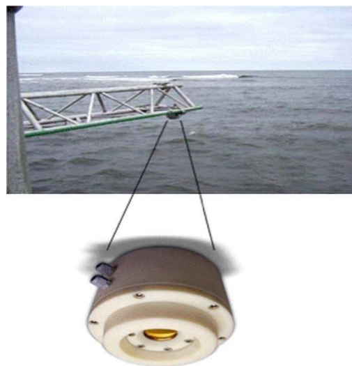
Figure 1: Ultrasonic sensor used to measure the height and time period of waves.
