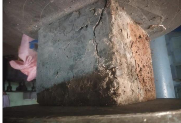
Figure 2: Testing cube for compressive strength
